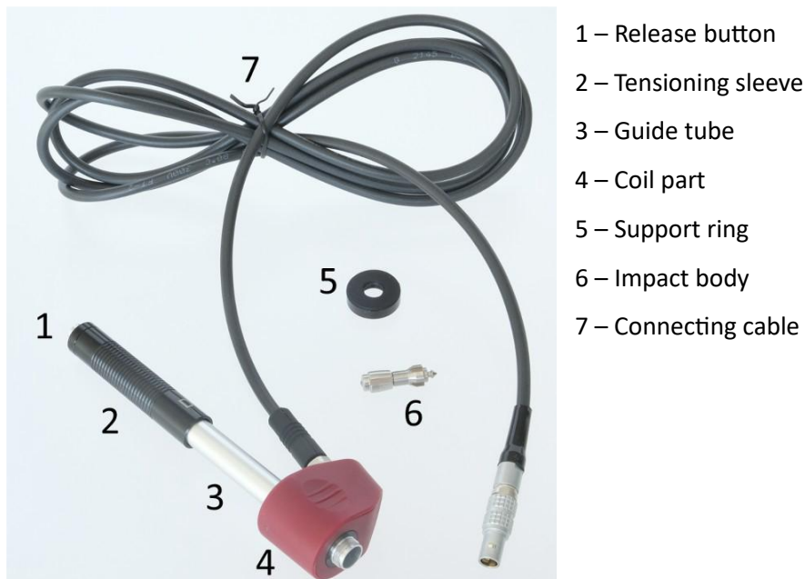
Fig. 26: Components of impact device type D
