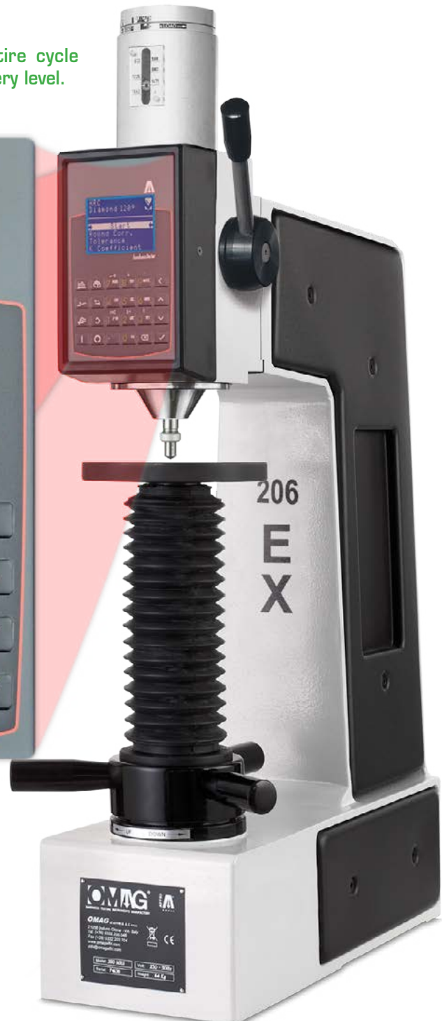
Touch key pad board IP 64 protection
