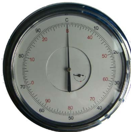
Figure 6-1 Zero the Scale
