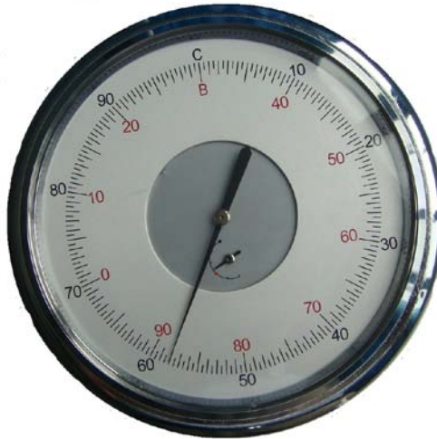
Figure 6-4 Read the Hardness Value
