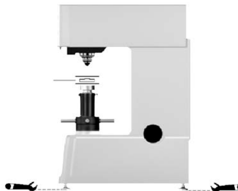
Figure 3-4 leveling the machine
