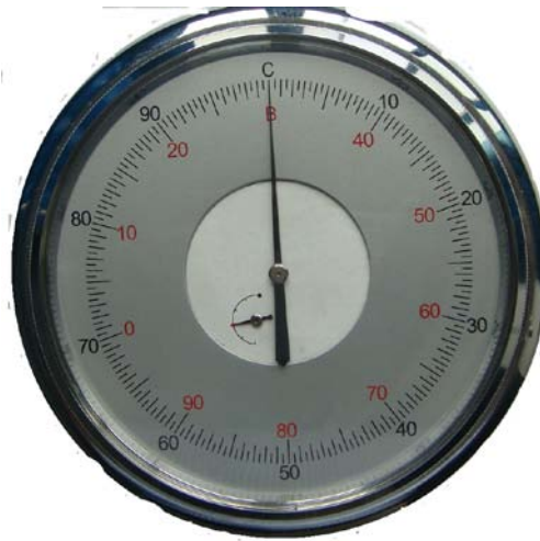
Figure 6-2 Small needle points to the red mark
