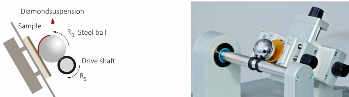
Image 1: Measuring principle of the calotte grinding method
