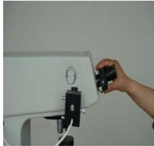
**Figure 3-4 Install Measuring Microscop**
