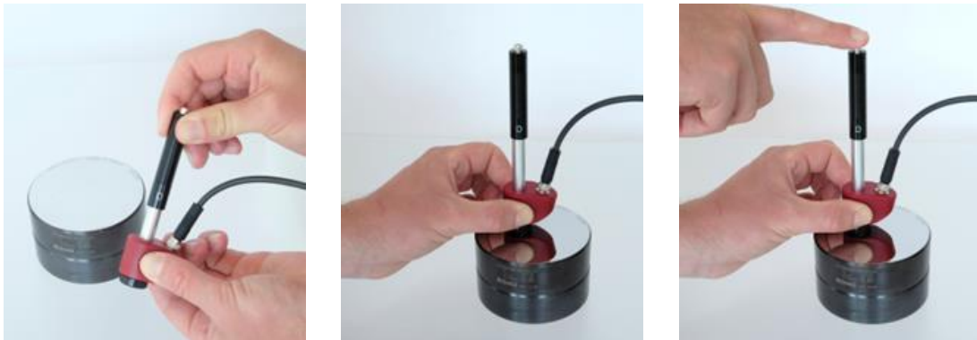
Fig. 13: Test with impact device type D
