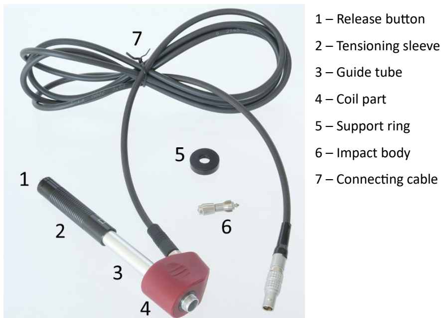
Fig. 12: Components of impact device type D
