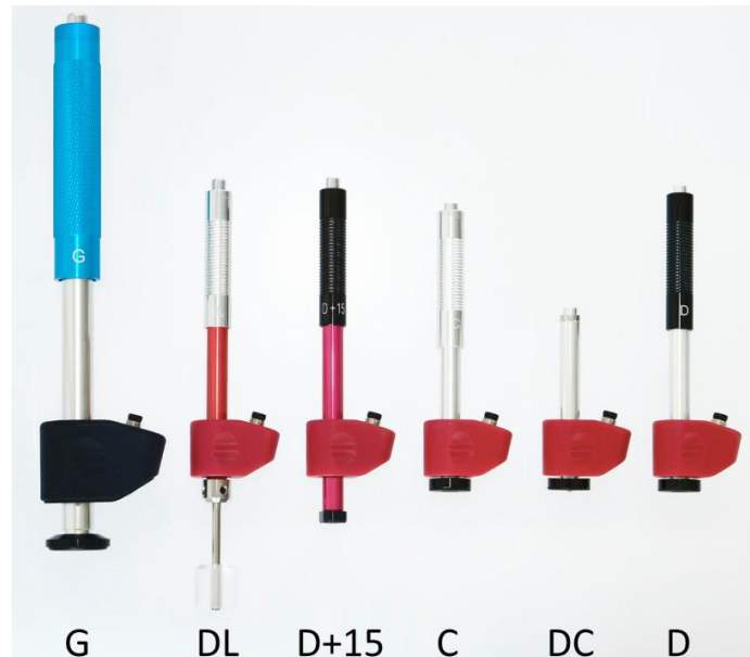
Fig. 3: Impact devices for hardness tests acc. to Leeb
